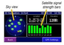
The sky view shows the satellites you are receiving. The satellite signal strength bars indicate the strength of each satellite signal. A solid bar indicates your Navigator III has a strong fix on that GPS satellite, and the GPS satellite is ready for use. For more information about GPS, see www.garmin.com/aboutGPS. See page 19 for information about the GPS Settings.
